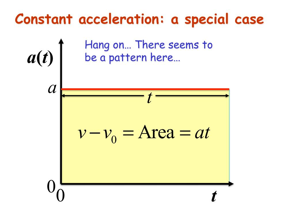
Constant acceleration: a special case It is rigorously true (a mathematical fact):  $v - v_0 =$  Area under a(t) curve = at  $x - x_0 =$  Area under v(t) curve  $= v_0 t + \frac{1}{2}at^2$ What we have discovered here is integration or calculus...
